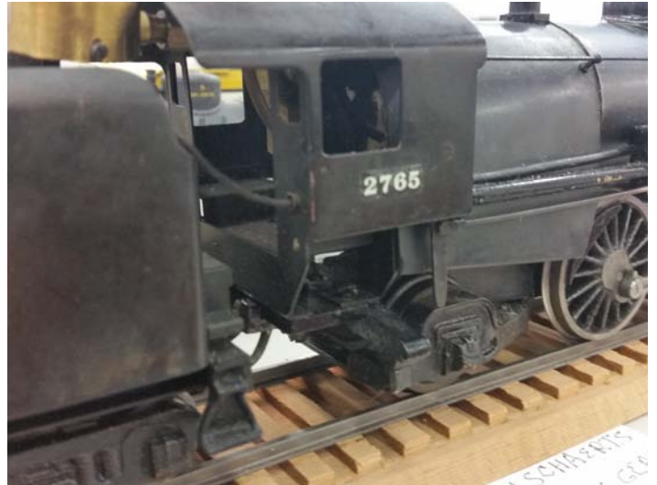
Below the cab you can see the actual working Walschaerts Valve Gear handle to control speed and direction
