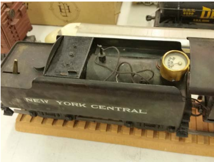
The tender appears to hold "white" gas which was a popular liquid fuel. The handle near the rear of the tender pressurized the fuel tank
