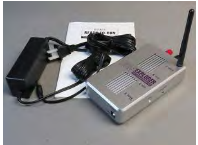
DCS Explorer and power supply. Notice that the wall transformer plugs into the Explorer Track Interface Unit, and the TIU into the track.
