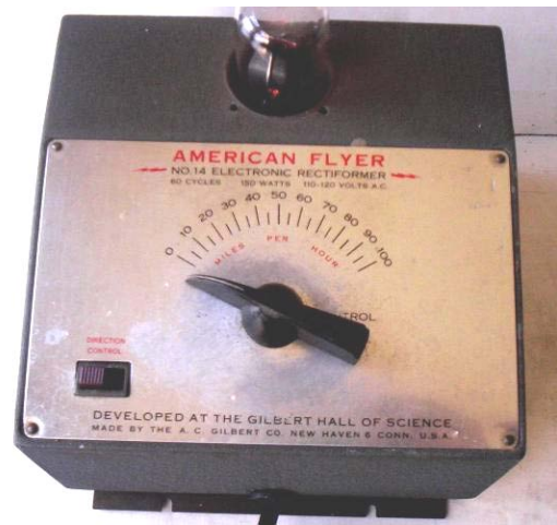
American Flyer's "Rectifier" the vacuum tube, missing it's wire safety shield, is at the top
