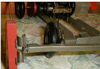
The 1928 model Electricar had sliding pick-ups along a fence with steel rails.
