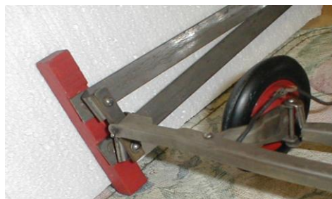
The 1928 model Electricar had sliding pick-ups along a fence with steel rails.
