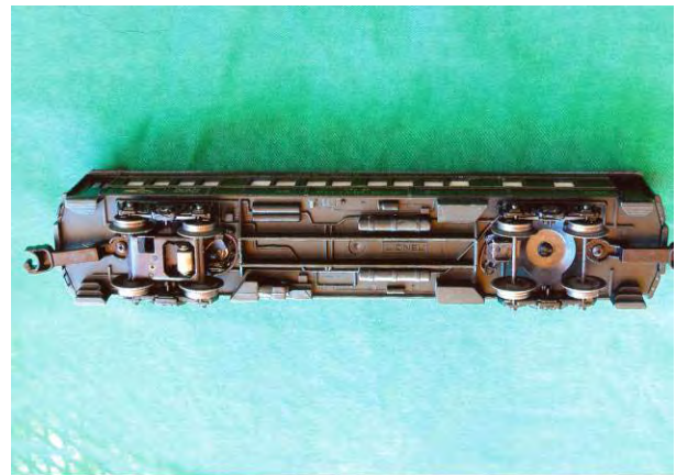
The underside of the 1984 Pittsburgh Convention Car showing fixed couplers and four wheel trucks
