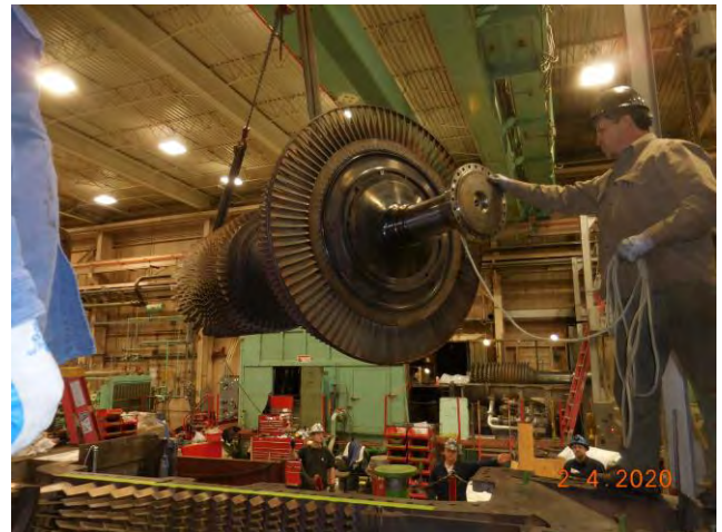
Turbine going back in and getting ready for reassembly
